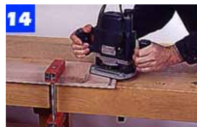
Clamp each drawer front to the workbench, and then use a router and dovetail bit to cut the dovetail dados.
