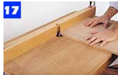
Install a straight bit in the router table, and then slide the door panel over the bit to cut the rabbet on the inside panel edges.
