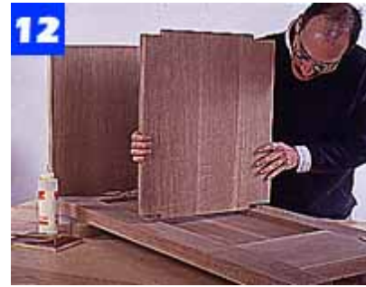
Apply glue to the slots, dowel holes, joining plates and dowels, then assemble the shelves to one case side.
