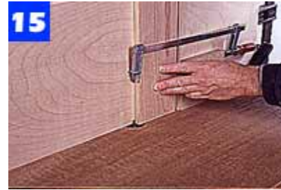
Cut the drawer side's dovetail in the router table. Clamp a backup block to the side, then move the side over the bit.
